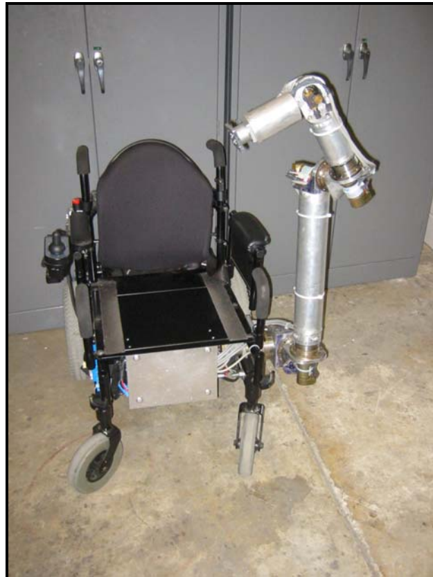
Figure 4.2: Completed Arm on Power Chair
