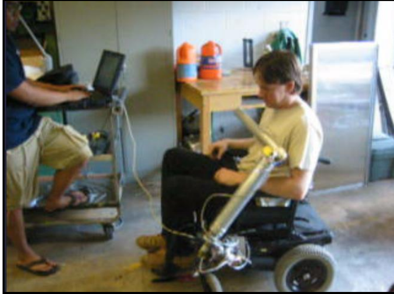
Figure 5.1: Automatic Shutdown when Force Limit is Exceeded
